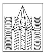
One way to tell when it's time for new tires is to check the treadwear indicators, which will appear when your tires have only 1/16 inch (1.6 mm) or less of tread remaining. You need a new tire if any of the following statements are true:
